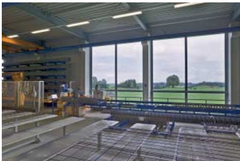
Fig. 6 At the second level – above the shuttering robot – the steel processing unit is located. Mats are welded just in time and exactly to specification.
