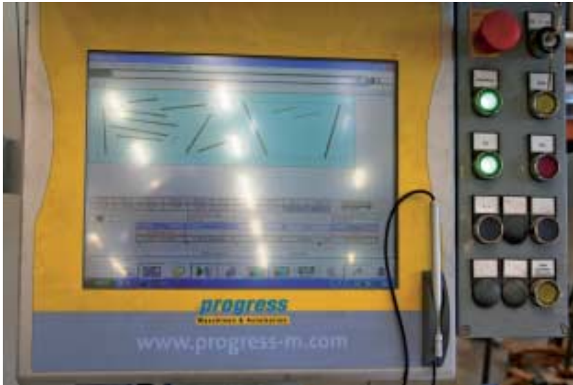
Fig. 5 A screen next to the robot displays the molds detected during the scan, which are then lifted by the robot.
