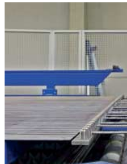
Fig. 6 At the second level – above the shuttering robot – the steel processing unit is located. Mats are welded just in time and exactly to specification.
