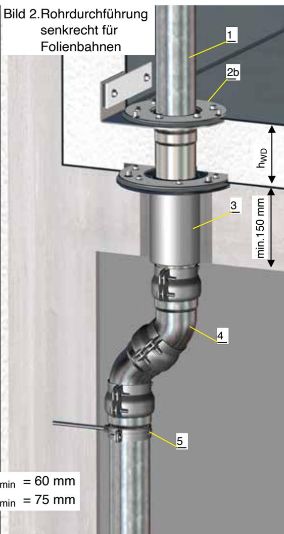
DN 70:  $h_{WD \min} = 60 \text{ mm}$
