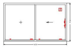
Product: WICSLIDE 65 Opening type: npd Area: 2.40 m<sup>2</sup> Transparent area: 1.73 m<sup>2</sup> Surface treatment: powder coating / anodized
