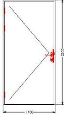
Product: WICSTYLE 65 Opening type: npd Area: 2.42 m<sup>2</sup> Transparent area: 1.64 m<sup>2</sup> Surface treatment: powder coating / anodized
