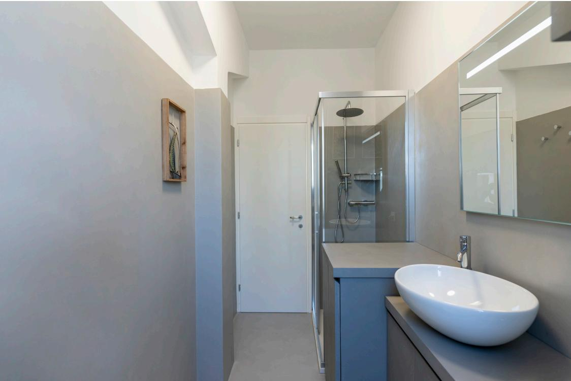
**EN** – Ideal Skin is used to create continuous and seamless surfaces on floors, walls and solid furnishings with an elegant, discreet and homogeneous design. It is applied by spatula in two coats with a total thickness of about 1,5 mm and is available in 16 basic colours that offer countless combinations.
