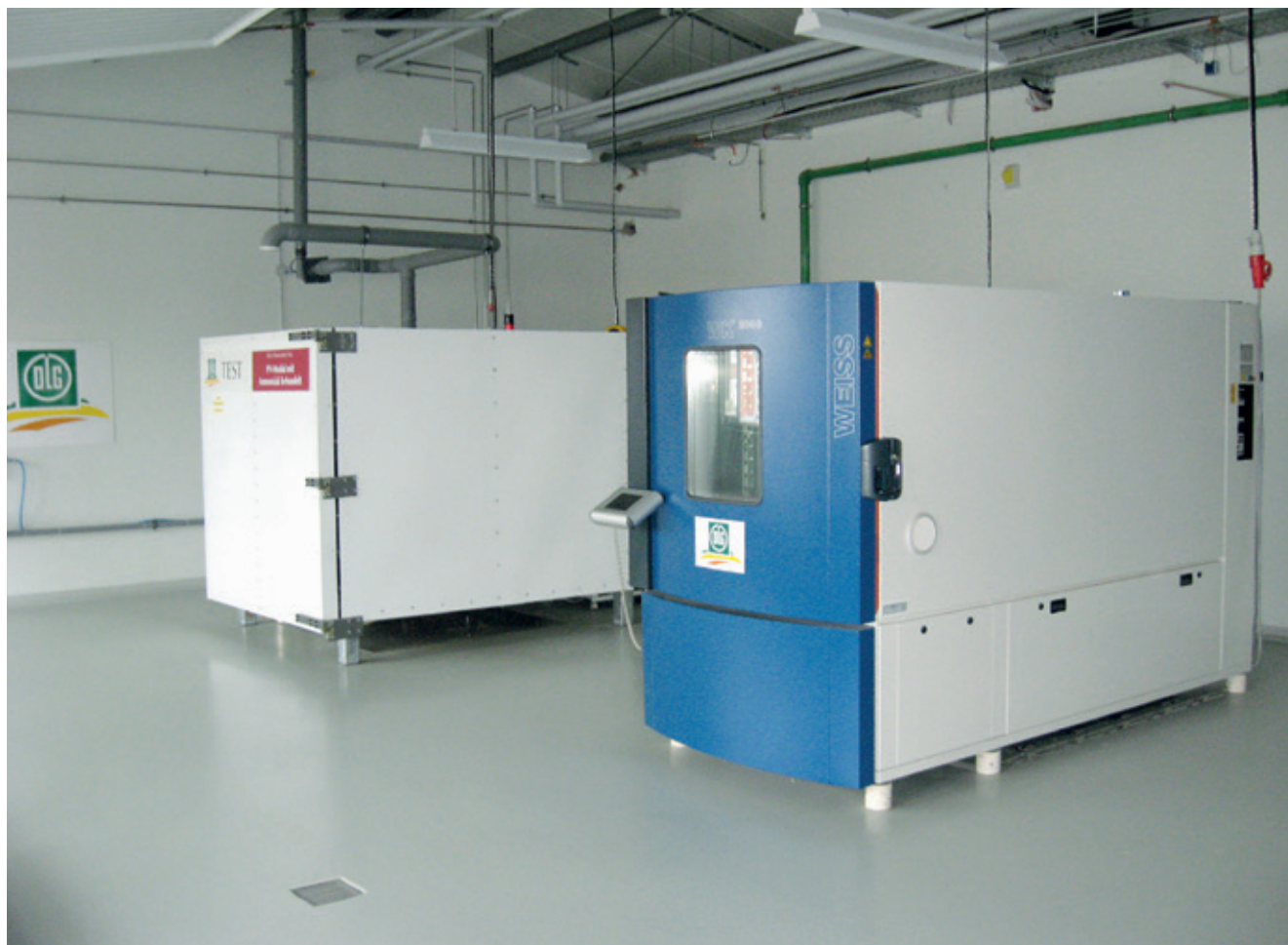
Figure 2: DLG test lab – two ammonia chambers
