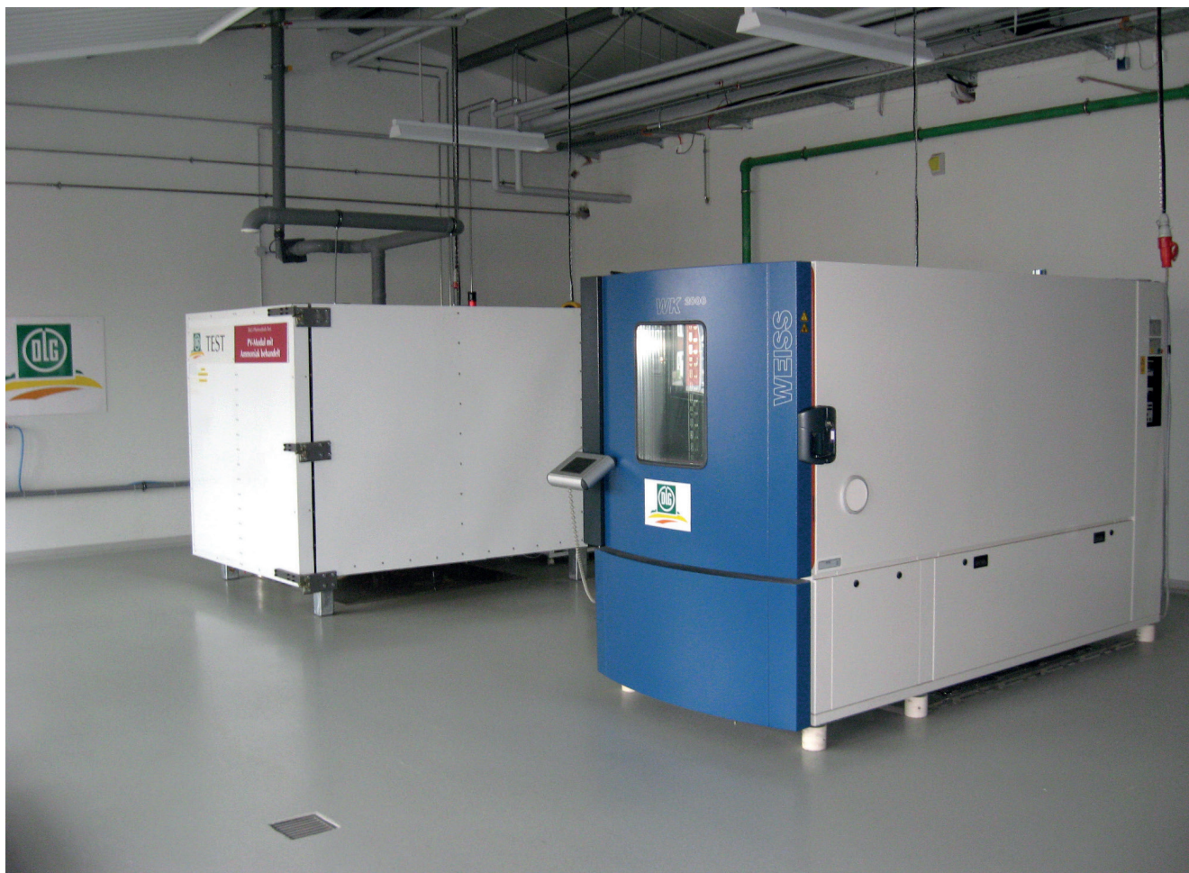
Picture 2: DLG test lab – two ammonia chambers
